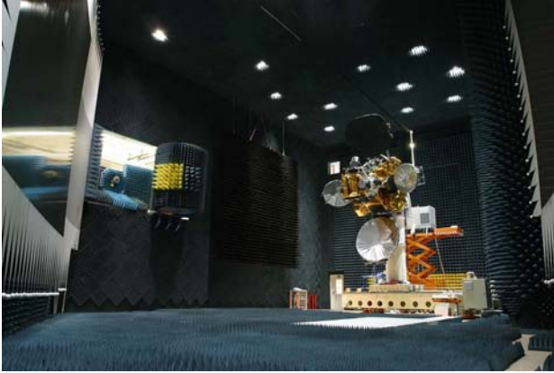
Figure 7-1: High-Power Side Wall in CCR
