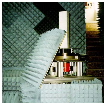
Figure 10 Mechanical Test Structure for RCS Measurements with Pylon, Positioner and Cover Plate; Lateral Positioner Absorber Plates Removed
