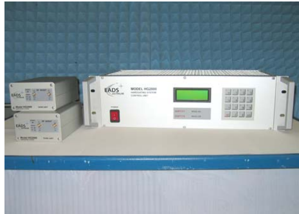
Figure 5 Hardgating System HG2000 of EADS Astrium with Control- and Tx-/Rx-Switch Units
