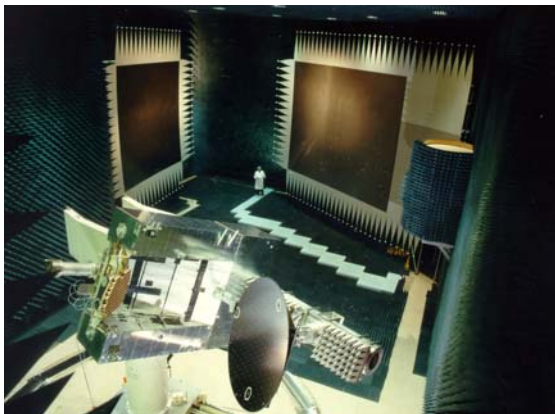
Figure 4 CCR 75/60 with INTELSAT VIII Multi-Feed, Reflector and Mockup Structure
