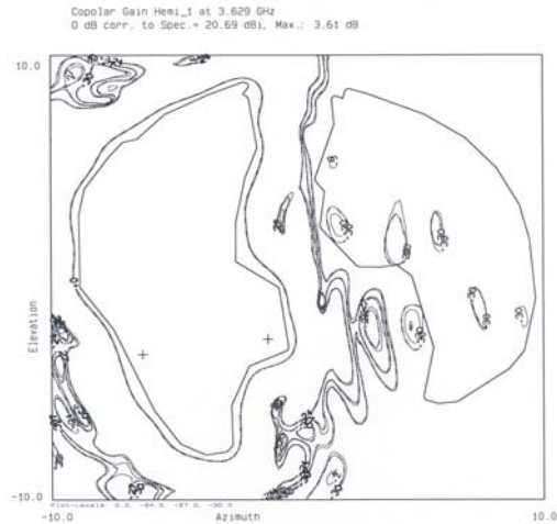
Figure 10: Overlay of the RF-Test Results of the Co-Polar Hemi 1 Beam, at Hot (+85°C, Solid) and Cold (-50°C, Dotted)
