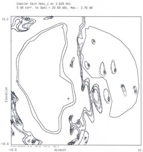
Figure 9: Overlay of the Pre- (Dotted) and Post Environmental (Solid) Test Results of the Hemi 1 beam Co-Polar Pattern
