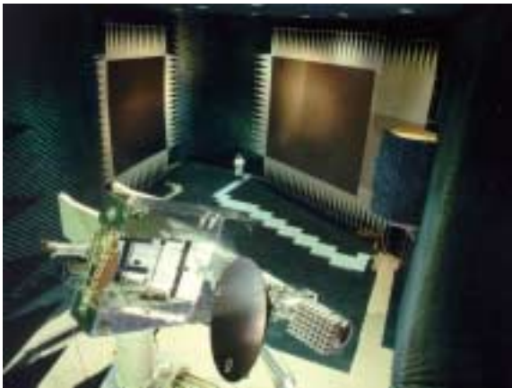
Figure 1 CCR 75/60 with Intelsat VIII Satellite Feed, Reflector and Mockup Structure
