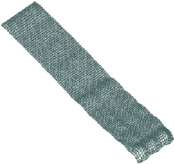
Figure 6 Enlarged Surface Distortions of two vertically placed Reflector Segments of the Main Reflector (Height of each Segment is 5 m)
