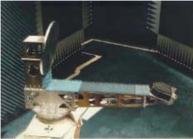
Figure 5 Highly Accurate Offset Reflector Antenna for Measurements up to 500 GHz as Representative Test Object (RTO) in the CCR
