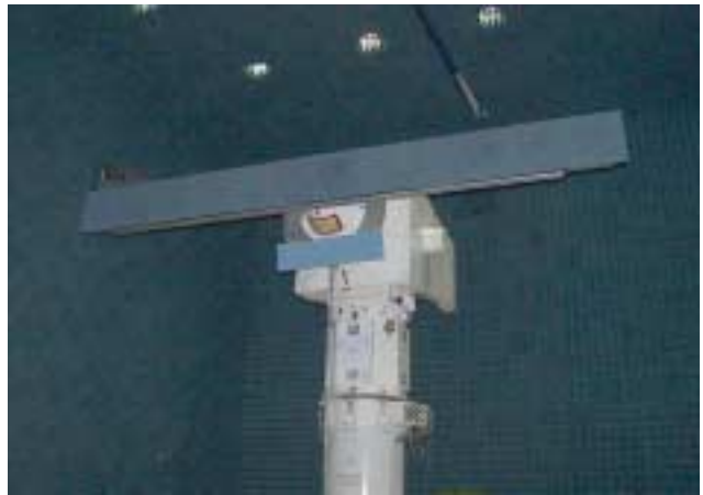
Figure 4 5 m Plane Wave Scanner of Astrium GmbH with 500 GHz Receive Module Mounted
